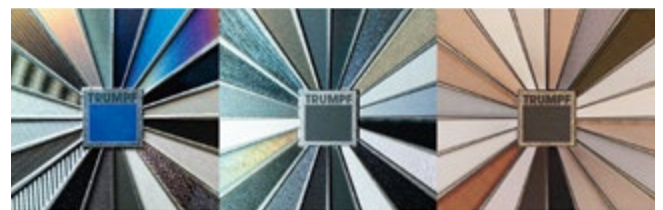
High-quality engraving in the watch industry: titanium (left), 316L (center), copper (right).
