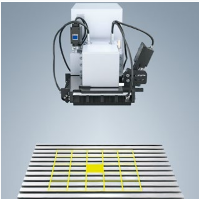
TRUMPF VisionLine facilitates the reading and evaluation of marking content on several processing levels.
